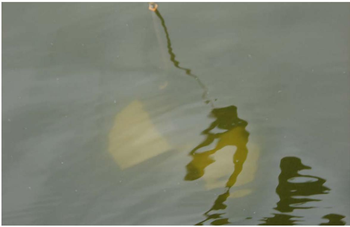
Photo 2: 29 May 2013 view of the secchi disk at a depth of 1 meter.
